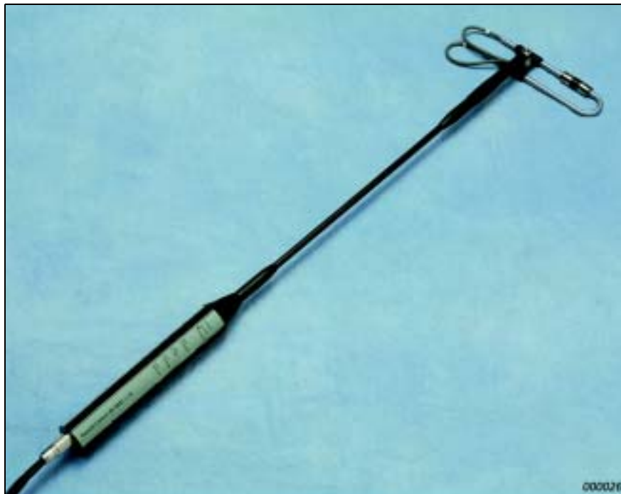
Fig. 2 The sound intensity probe consists of: Dual Preamplifier Type 2683 and Sound Intensity Microphone Pair Type 4197. Here you can see it placed on its extension stem
